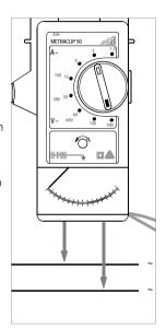
value, switch to a lower measuring range with higher resolution.
